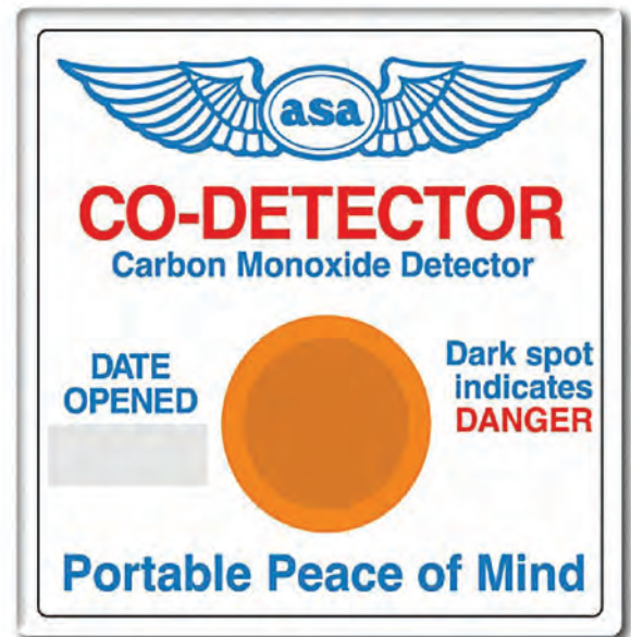
(Above) This is an example of a 'Dead Stop' CO warning card, which goes black in the presence of carbon monoxide. These cards are lifed, generally for no more than twelve months after opening, and some, once they've gone black, are no longer serviceable. Others, like this example from Aircraft Spruce and Specialty, return to their neutral colour once the CO presence has ceased and can continue to be used. Make sure you date the card and replace it when its life has expired.
